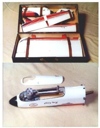
glass fibre. The fuselage is moulded 1/16 balsa covered in glass cloth inside and out. The undercarriage is plug in and made of titanium. The lead out tubes are springs and non-adjustable. The props are a very light hard wood (possibly lime wood) and essential to the effective running of the motor as are the sup-
