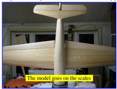
I now take the model out of the jig, remove the rods and put them to one side for use on another model. A check on the scales now to see how you are progressing – mine came out at 28 ounces which is in the ball park at this stage.
