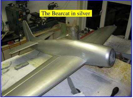
weight white tissue. Note, when you cover a model with fibreglass cloth and resin a further covering of tissue stops the weave of the cloth grinning through the finish.
