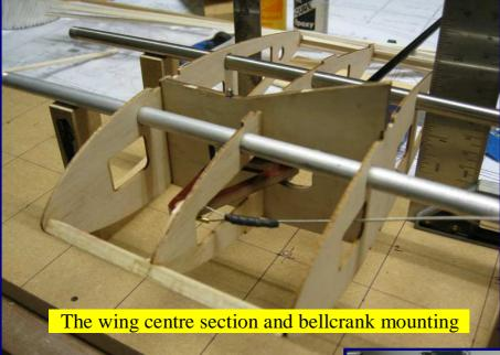
Before you can start building the wing you have to make up the centre section that carries the bellcrank mounting. Now this is fun, as two pairs of hands are needed to get it all aligned. The video suggests that you build the wing then put the bellcrank in and glue the main pivot pin in afterwards. but I wasn't convinced that was the best approach. You will have to decide for yourself.
