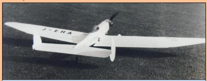
Stan's original 'Kentish Wind' built in 1952 and as used in demos. Powered originally by a PB Amco 3.5cc, but after several derivatives, finally fitted with a 5cc SR special.
